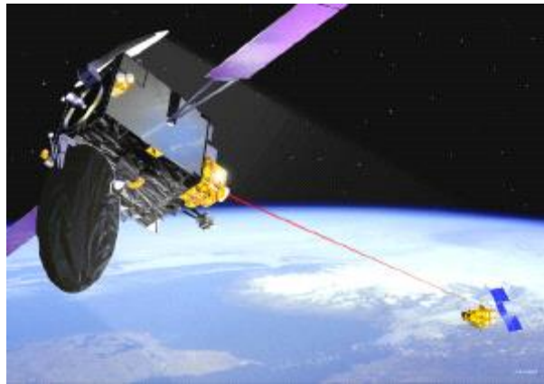
Figure 3.2. Communication between Spot and Artemis with Silex laser system
