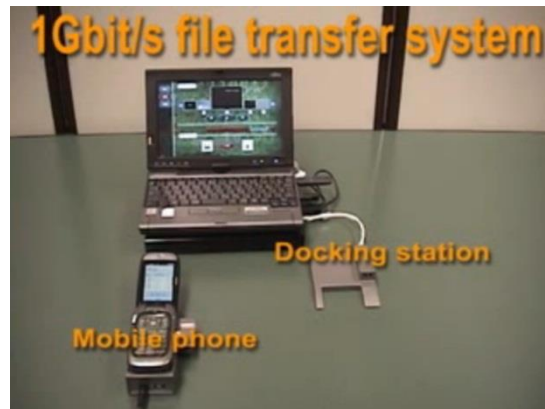
Figure 3.25. IrDA 1Gbps file transfer from Docking station to mobile phone
